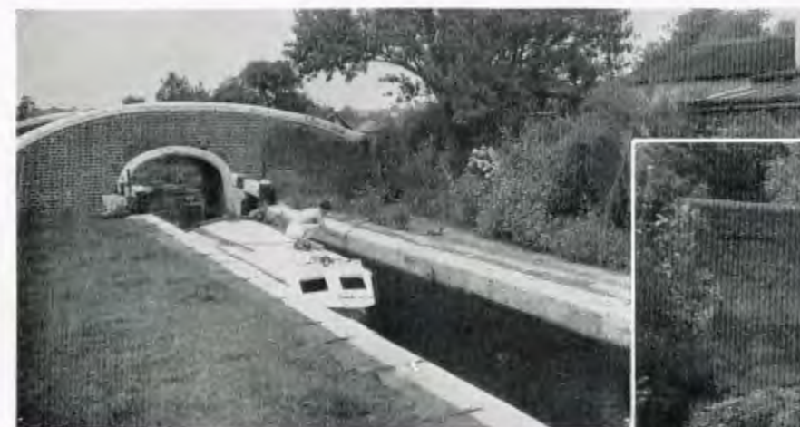
The converted airborne lifeboat negotiates the hazards of a canal lock and bridge. These lifeboats were slung beneath bombers like the Shackleton and dropped for the rescue of shot-down aircrews. The lifeboat shown here is the Mark 3, an aluminium vessel designed by Saunders-Roe
